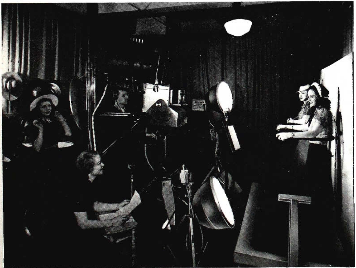
ACTION SHOT OF EARLY TELEVISION EXPERIMENT IN BLOOMINGDALE'S DEPARTMENT STORE. Fashion shows picked up from sixth floor studio were seen on wired receivers on third floor. Because of lack of sensitivity of early cameras, depth of focus obtainable was very restricted. This picture shows how models were forced to fit themselves into rigid arm and back supports in order to stay in focus. Note also they are standing on a sliding platform arrangement, which was used to push them before the camera and then pull them away. Camera was fixed in position. Post-war television, of course, will have none of these restrictions.
